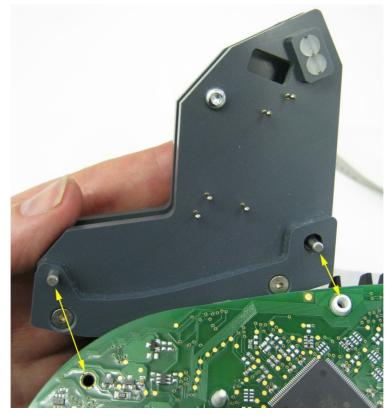
Try to avoid dragging the pins sideways over the PCB whilst aligning the pegs to the location holes.
