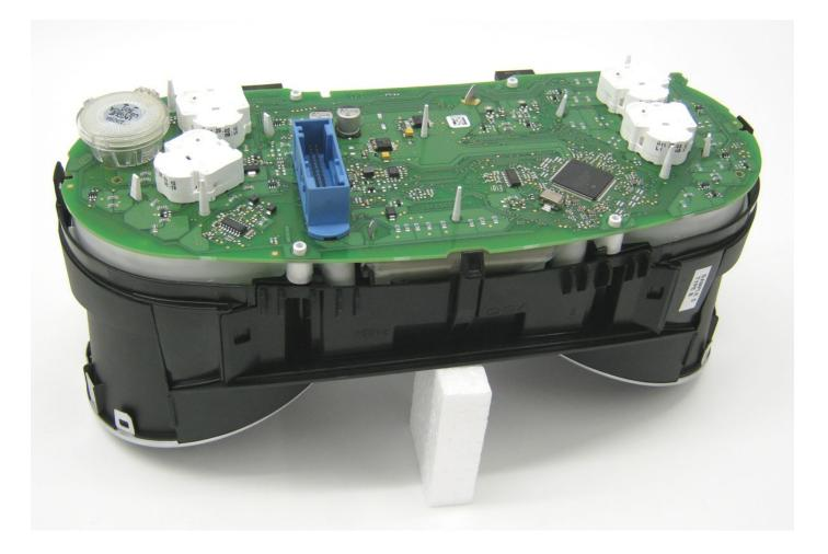
2) Remove the back cover of the instrument pack, and determine which type of PCB layout is present. Use the appropriate adapter.
